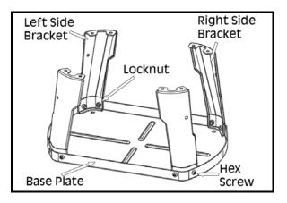
2. Install the seat chassis (2) on to the brackets (7 & 8). Lock the chassis in place using the socket head cap screws (4) and M6 locknuts (5)
